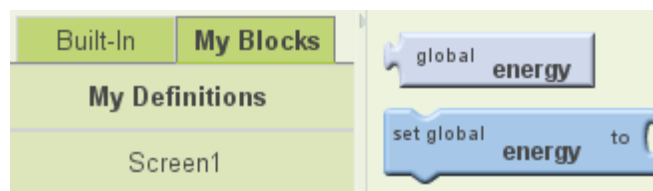
Figure 5-5. View of the My Definitions drawer showing new global energy and set global energy blocks
